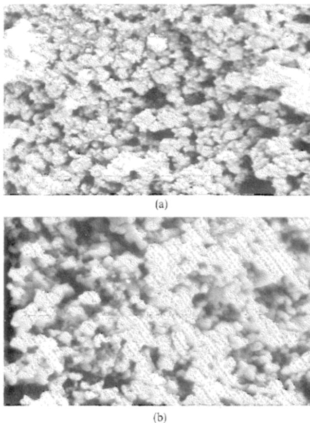
Fig. 2. Morphology of zinc oxide composite powder: (a) as flashed (original magnification  $\times 2000$ ); (b) after grinding (original magnification  $\times 4000$ ).
