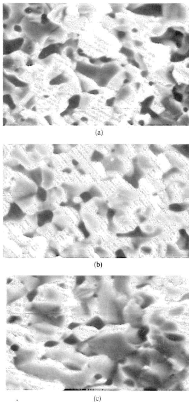
Fig. 3. Fractograph of doped zinc oxide sintered at  $1200^\circ\text{C}$ : (a)  $0.0\ \text{mol}\%$ ; (b)  $0.3\ \text{mol}\%$ ; (c)  $0.5\ \text{mol}\% \text{K}_2\text{O}$ . (Original magnifications  $\times 4000$ ).
