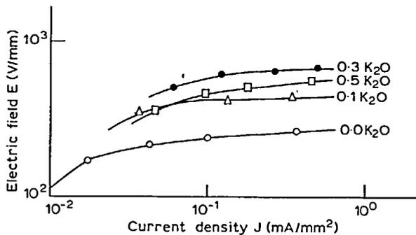
Fig. 4. Current density vs electric field of Pr doped ZnO varistor prepared by flash decomposition method.
